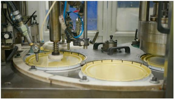
The one-component sealant system Darex COV 73 is suitable for nozzle application, offering stable viscosity, high resistance to solvents, ketones and oils, and thermal stability.
